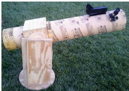
**Anybody want an awesome telescope?** – Have you ever considered making your own? Using a set of commercial mirrors and material readily found at most hardware stores, you can build your own telescope with performance surpassing most store bought instruments. Contact the club for more info.
